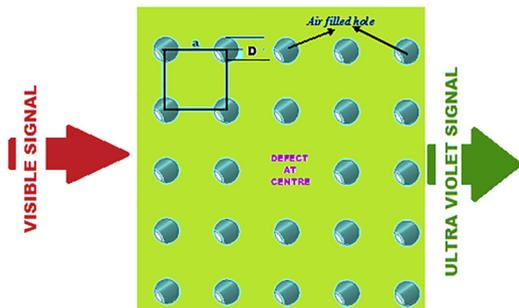
Fig. 2. Cross-sectional view of square type photonic crystal fiber.
