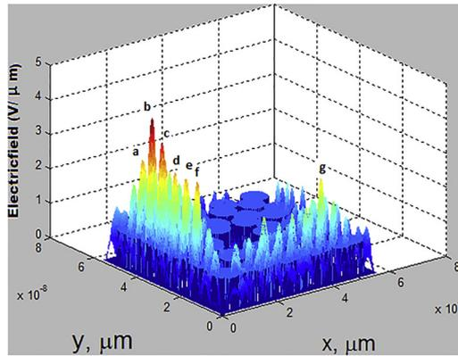
Fig. 3. Electricfield distribution in photonic crystal fiber.
